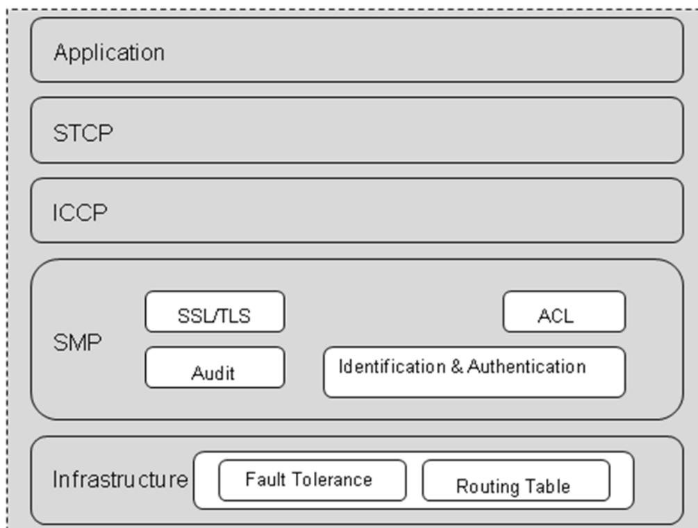
The specific functionality detailed in the white boxes is executed in a distribute way. The modules SSL/TLS, ACL, Audit, Identification & Authentication and Fault tolerance are executed in the OMU board. The modules relating with the routing table and connection filtering out of the management network are executed on the interface board.
